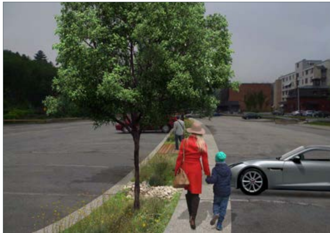
▲ RETROFIT OPPORTUNITY: The same parking lot retrofitted with a vegetated swale median placed between parking stalls. Specific design considerations should be taken to manage pedestrian flow through these landscape areas.
