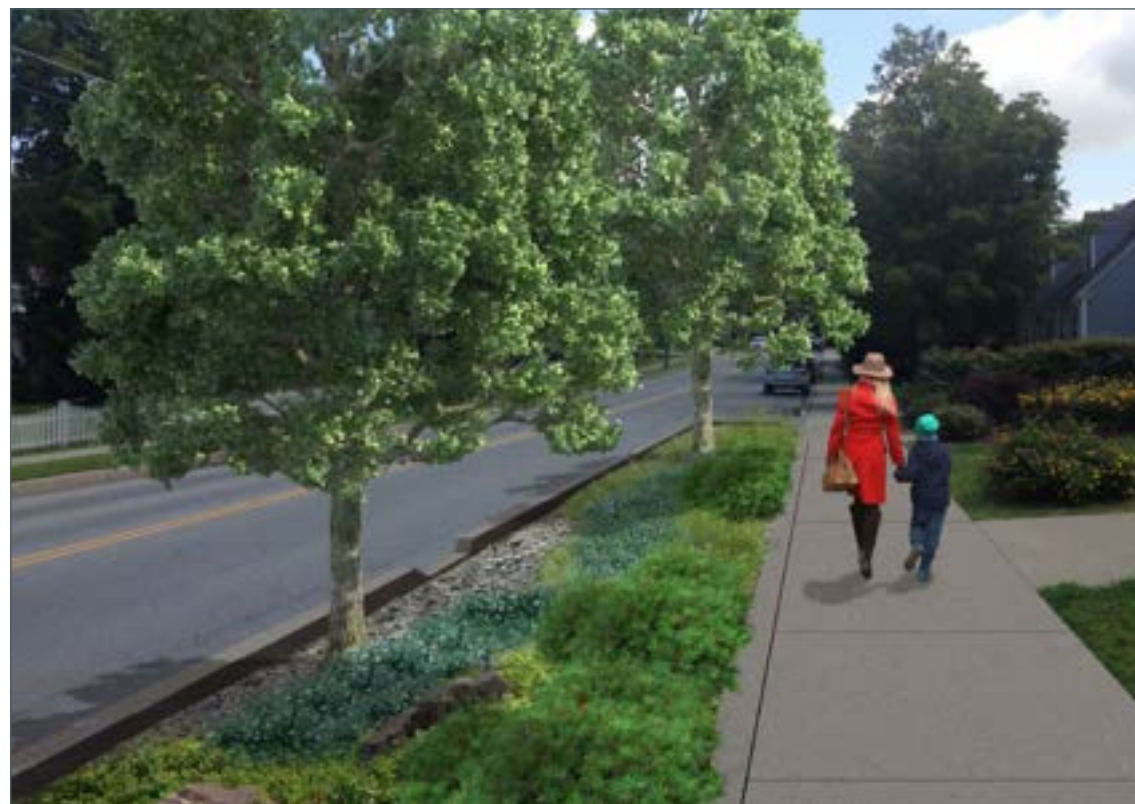
▲ RETROFIT OPPORTUNITY: The same arterial street retrofitted with a stormwater curb extension.
