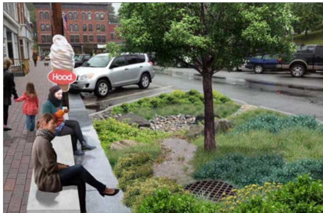
▲ RETROFIT OPPORTUNITY: The same downtown main street retrofitted with stormwater curb extension. In this example, the stormwater curb extension also uses space that is already striped as “no parking”.
