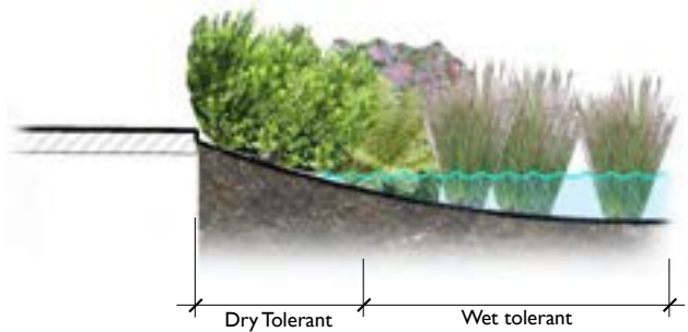
Typical Side Slope and Flat-Bottom Planting Condition
